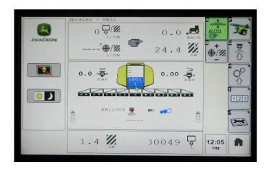
Note: Do not power down this display by removing battery power. If this has been done 10 times, the display will crash, and only AMS factory can run an update. The counter will be reset after a proper power down via ignition switching.
